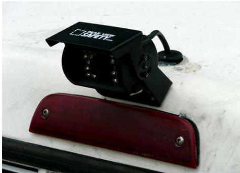
Figure 5. Camera mounted just above top rear brake light.
