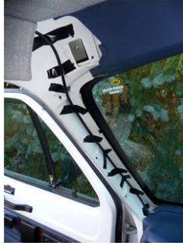
Figure 9. Run the camera cable down the A-pillar and secure it with electrical tape.
