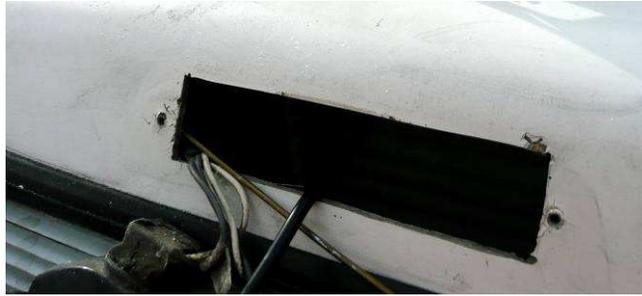
Figure 2. Top brake light hole allows cable fishing from inside.
