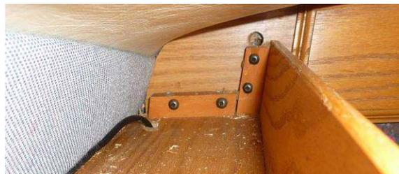
Figure 8. Camera cable runs down through tray front into A-pillar behind cloth trim.
