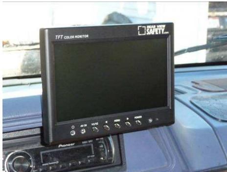
Figure 10. Monitor is mounted on dashboard with minimal view obstruction.
