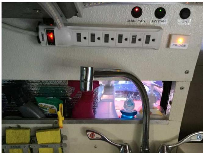
We found that we wanted to leave the fans on because the lighted switch showed us that the fridge was running, so we installed an LED light (like we did for the furnace and the water heater so we would know when they were turned on). The amber LED is quite bright and actually makes a good night light for the bathroom.
