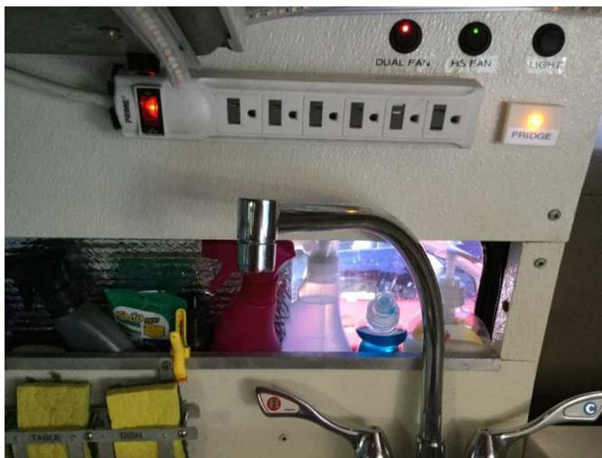
We found that we wanted to leave the fans on because the lighted switch showed us that the fridge was running, so we installed an LED light (like we did for the furnace and the water heater so we would know when they were turned on). The amber LED is quite bright and actually makes a good night light for the bathroom.
