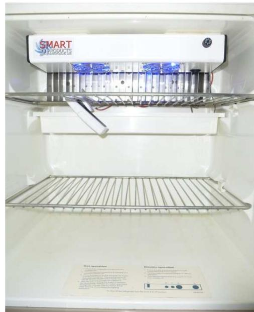
After about six months we can say that the Fridge-Fix fan definitely prevents ice buildup on the fins. We never find water in the catch tray after use any more. And we have used it in very humid environments.
